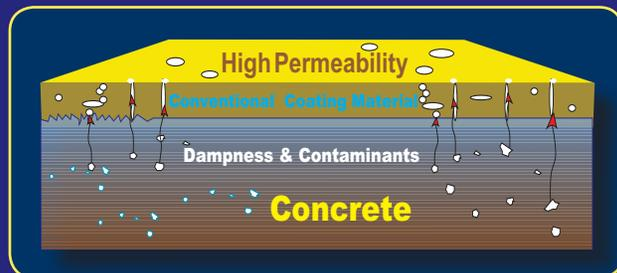
**Conventional coatings (and so-called liquid applied "linings") will always have severe problems with permeability when field applied.**
